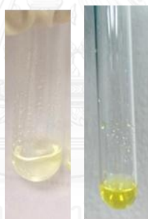
Figure 4.7 Photograph of Ellman' reagent test of before (left) and after (right) ring opening of the dithiol group in thiotic acid
