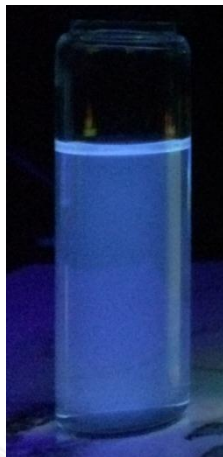
Figure A1 The photograph of ZnSe/ZnS QDs under a black light lamp
