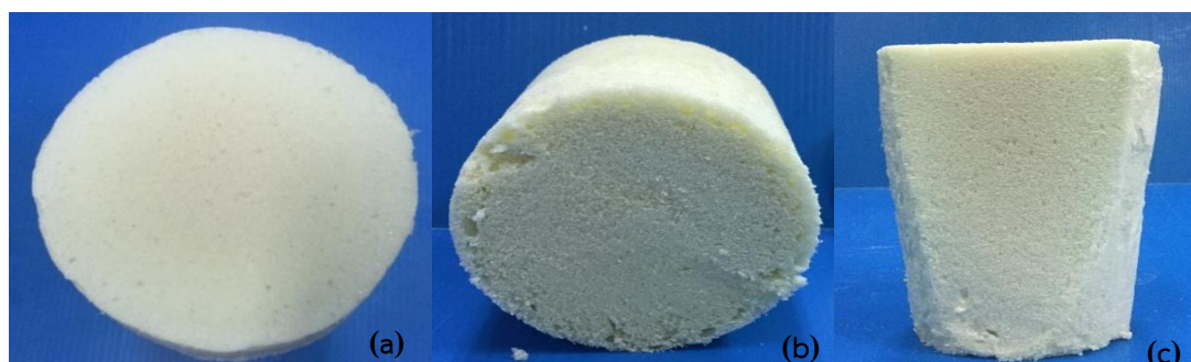
Figure 4.47 RPUR foams catalyzed by \text{Cu}(\text{OAc})(\text{Ala}) (1:2); the amount of catalyst = 1 pbw and the amount of blowing agent ( \text{H}_2\text{O} ) = 4 pbw.
