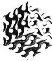
Figure 2.7 Pore model of 3-D cubic mesoporous mesostructure with symmetry of Ia3d (Lu et al. , 2009).
