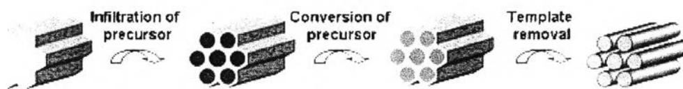
Figure 2.11 The illustration of nanocasting pathway (Lu et al. , 2009).
