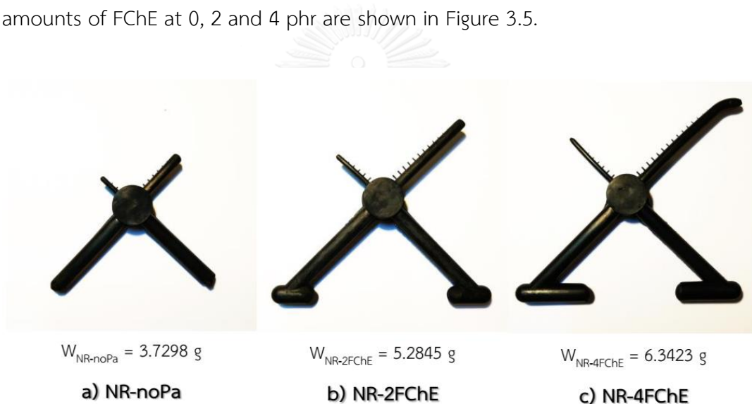
Figure 3.5 Spider mold specimens and their average weight of a) NR-noPa, b) NR-2FChE and c) NR-4FChE
