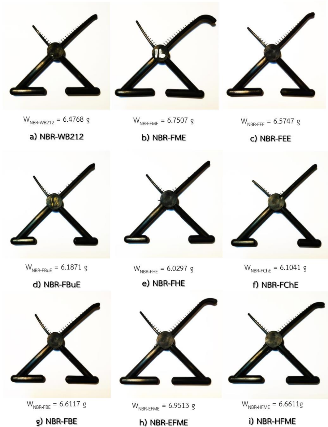
Figure 3.6 Spider mold specimens and their average weight of a) NBR-WB212, b) NBR-FME, c) NBR-FEE, d) NBR-FBuE, e) NBR-FHE, f) NBR-FChE g) NBR-FBE, h) NBR-EFME and i) NBR-HFME
