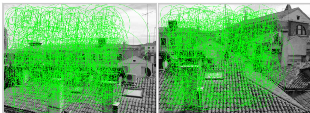
(c) Detected features in image1 using SIFT (d) Detected features in image2 using SIFT
