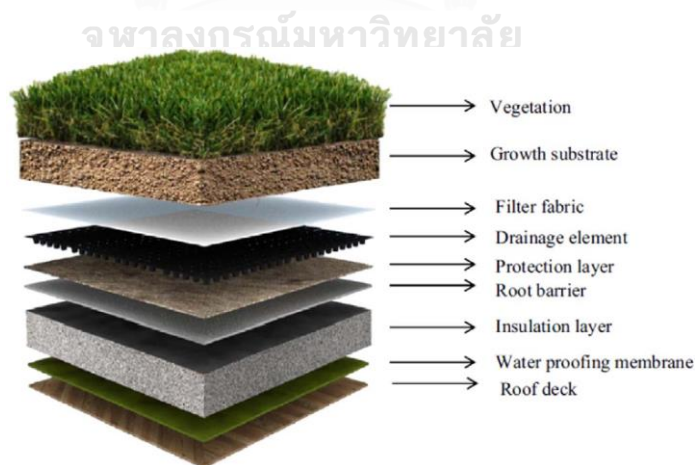
Figure 2.1 Green roof structure
