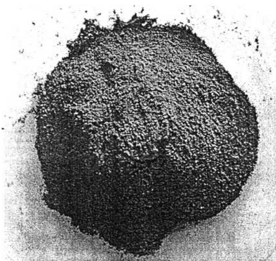
Figure 4.1 The sludge from the Metropolitan Waterworks Authority.
