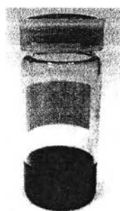
Figure 3.3 A CSA doped PANI solution
