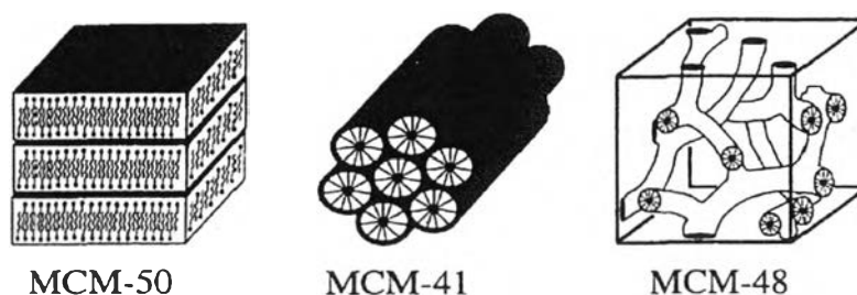
Figure 2.1 Schematic diagram of the M41S materials, MCM-50 (layered), MCM-41 (hexagonal) and MCM-48 (cubic) [20].
