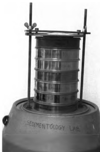
Figure 3.6 A mechanical shaker used for sieve analysis
