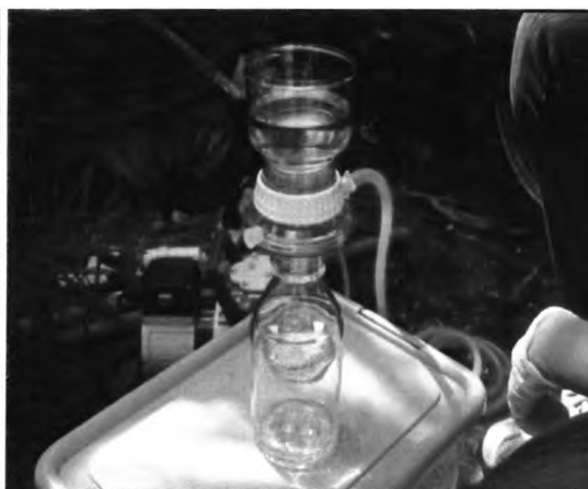
Figure 3.4 Field filtering of water samples
