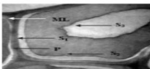
[ML-middle Lamella, P-Primary Wall, S1, S2, S3- Secondary cell wall sub layer]
