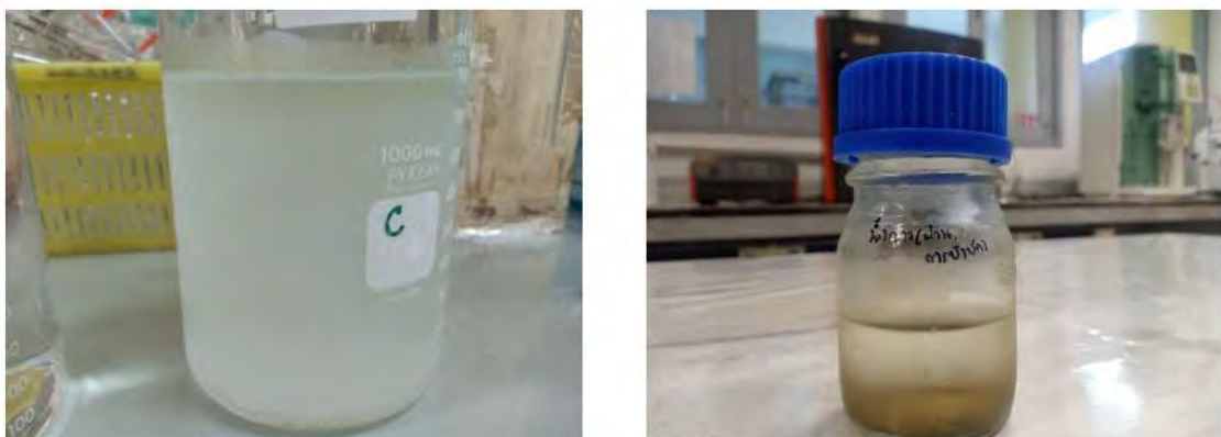
Figure 3.5 WAUF wastewater before and after treatment via Fe 0 /air modified Fenton reaction
