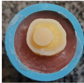
Figure 8 . ZLS disc cemented to dentin specimen.
