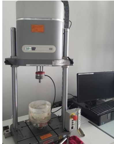
Figure 11. Universal Testing Machine (E1000, INSTRON instruments)
