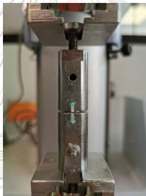
Figure 4 Tested microtensile specimen mounted onto a universal testing machine (EZ-S; Shimadzu Corporation, Kyoto, Japan)
