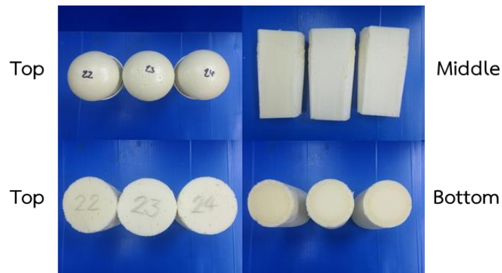
Figure 4.27 PIR foam catalyzed by DMCHA:K-15 = 0.5:3.0, water 4 pbw and NCO index =160
