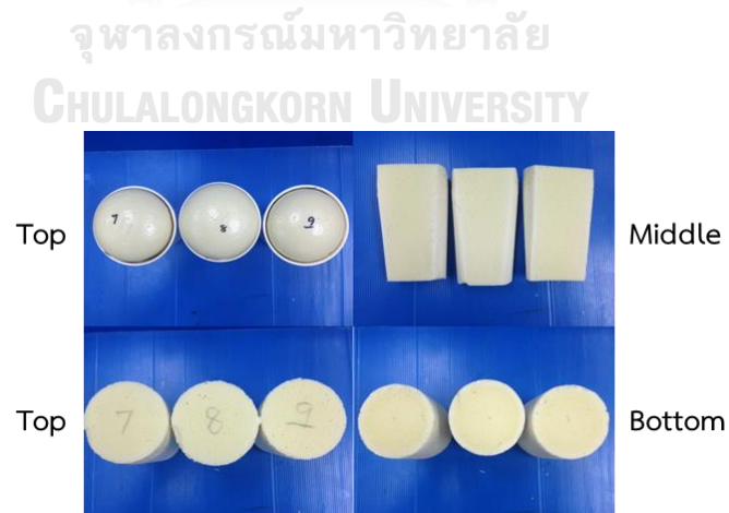
Figure 4.7 PIR foam catalyzed by DMCHA:K-15 = 0.5:2.0, water 3 pbw and NCO index =200
