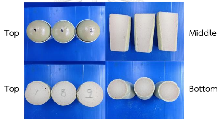
Figure 4.38 PIR foam catalyzed by \text{Cu}(\text{OAc})_2(\text{trien})\text{:K-15} = 0.5\text{:}3.0 , water 5 pbw and NCO index = 250
