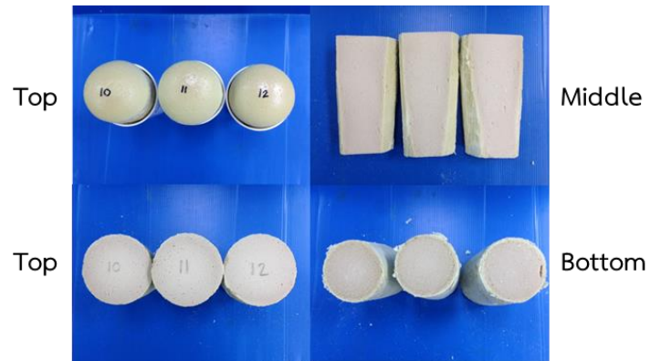
Figure 4.37 PIR foam catalyzed by \text{Cu}(\text{OAc})_2(\text{trien})\text{:K-15} = 0.5\text{:}3.0 , water 5 pbw and NCO index = 200
