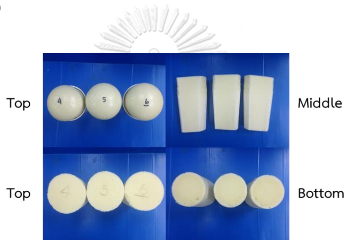
Figure 4.10 PIR foam catalyzed by DMCHA:K-15 = 0.5:2.0, water 4 pbw and NCO index =200
