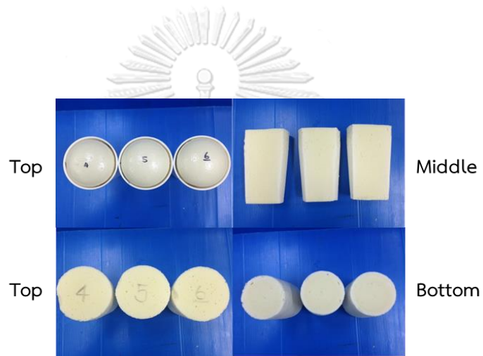
Figure 4.7 PIR foam catalyzed by DMCHA:K-15 = 0.5:2.0, water 3 pbw and NCO index =200
