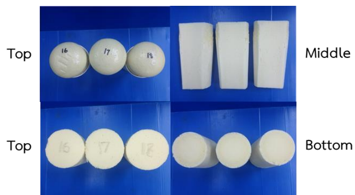
Figure 4.20 PIR foam catalyzed by DMCHA:K-15 = 0.5:2.5, water 4 pbw and NCO index =250
