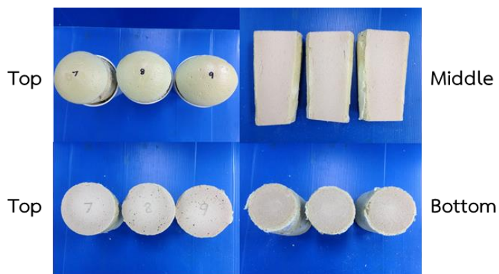
Figure 4.34 PIR foam catalyzed by \text{Cu}(\text{OAc})_2(\text{en})_2:\text{K-15} = 0.5:3.0 , water 5 pbw and NCO index = 200
