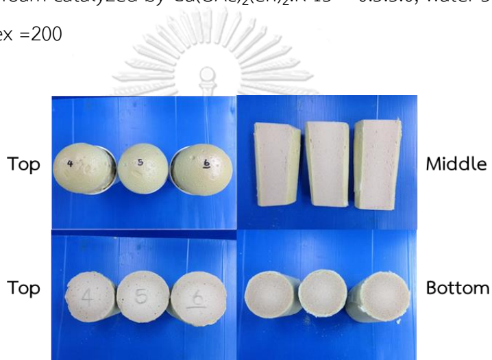
Figure 4.35 PIR foam catalyzed by \text{Cu}(\text{OAc})_2(\text{en})_2:\text{K-15} = 0.5:3.0 , water 5 pbw and NCO index = 250
