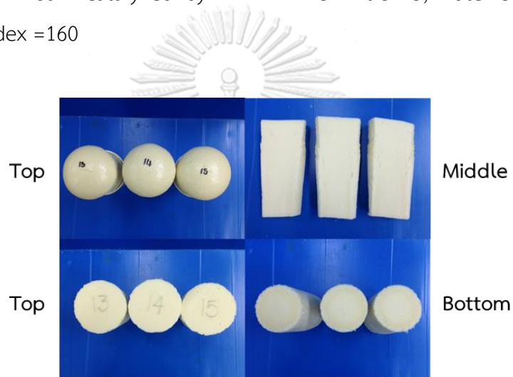
Figure 4.22 PIR foam catalyzed by DMCHA:K-15 = 0.5:2.5, water 5 pbw and NCO index =200
