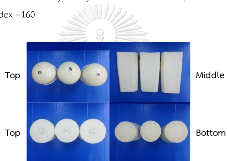
Figure 4.19 PIR foam catalyzed by DMCHA:K-15 = 0.5:2.5, water 4 pbw and NCO index =200
