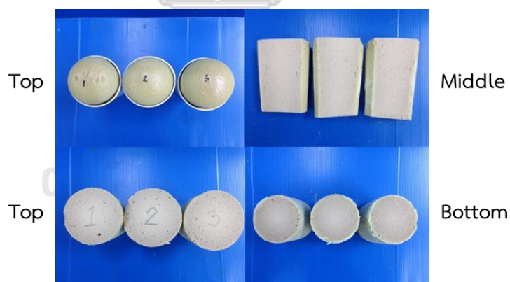
Figure 4.33 PIR foam catalyzed by Cu(OAc) 2 (en) 2 :K-15 = 0.5:3.0, water 4 pbw and NCO index = 250
