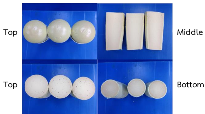
Figure 4.39 PIR foam catalyzed by \text{Cu}(\text{OAc})_2(\text{EA})_2:\text{K-15} = 0.5:3.0 , water 5 pbw and NCO index = 200
