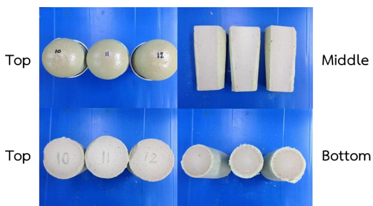
Figure 4.36 PIR foam catalyzed by \text{Cu}(\text{OAc})_2(\text{trien}):\text{K-15} = 0.5:3.0 , water 4 pbw and NCO index = 250
