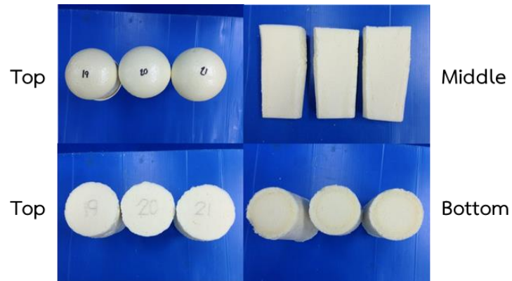
Figure 4.30 PIR foam catalyzed by DMCHA:K-15 = 0.5:3.0, water 5 pbw and NCO index =160
