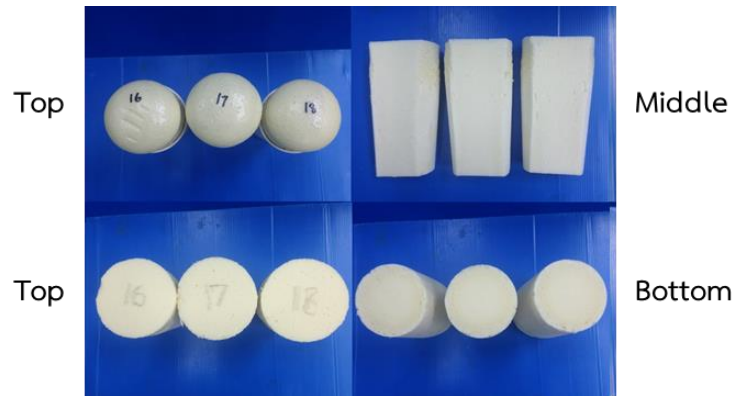
Figure 4.15 PIR foam catalyzed by DMCHA:K-15 = 0.5:2.5, water 3 pbw and NCO index =160
