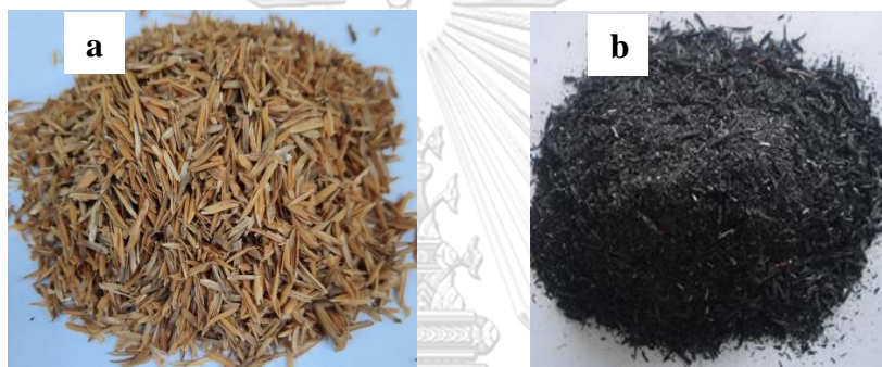
Figure 3. 2 Rice husk (a) and black rice husk ash (b) from rice milling plant
