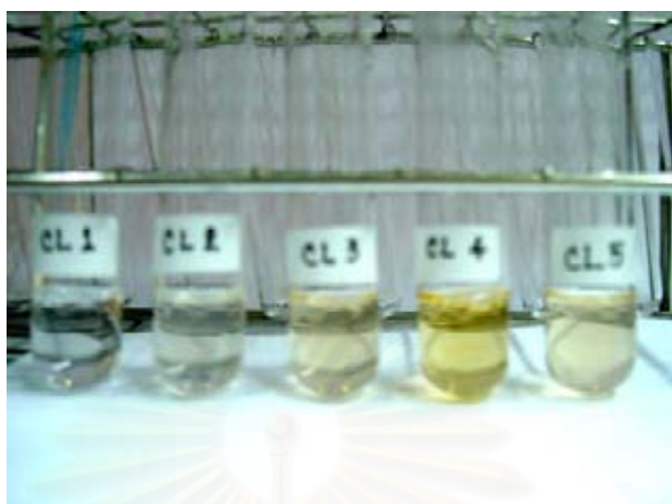
Figure I-12 Lycopene loaded chitosan coated liposome nanoparticle suspensions after centrifuge at 3,500 rpm for 1 h at 4°C. CL1-5 is prepared from the initial lycopene concentration of 45.75, 88.98, 140.56, 200.28 and 234.16 \mu\text{g/mL} , respectively.
