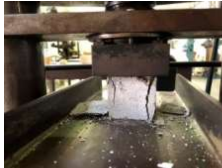
Figure 4.7 Compressive strength test
