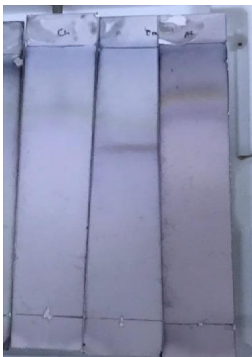
Figure 3.1 TLC analysis results of three pesticide standards (100 ppm each) with 40 \mu L of the loaded volume: chlorpyrifos, carbaryl, atrazine from left to right, respectively
