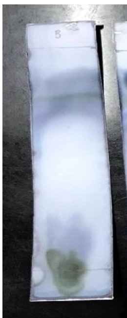
Figure 3.3 TLC analysis result of the bee pollen sample with 40.00 \mu\text{L} of the loaded volume
