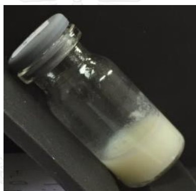
Figure 4.5 Appearance of hydrogel of 4 wt% SF induced by oleic acid-poloxamer surfactants
