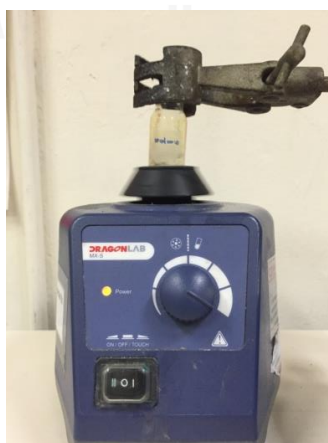
Figure 3.4 A vial of silk fibroin solution attached with a holder being vortexed
