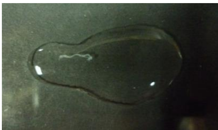
Figure 4.3 Sterilization of 1 wt% SF solution by sterile filtration. The appearance of resultant filtrate demonstrated mixed solution and white gel strips
