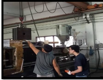
Figure 14: Researcher try to install mold into injection machine
