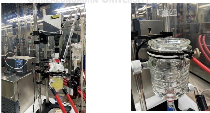
Figure 14 1-L double jacket reactor.
