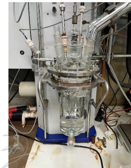
Figure 13 Automatic reaction calorimeter (RC1e, Mettler Toledo)
