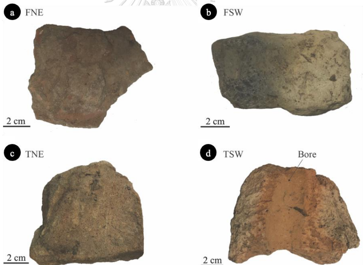
Figure 4.2 Photographs of the samples: (a, b) furnace fragments (a) FNE and (b) FSW and (c, d) the tuyère samples (c) TNE and (d) TSW.
