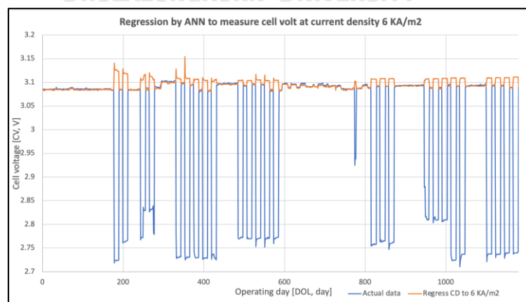
Figure 46 ANN model fitting in predictive CV after at CD 6 \text{ KA/m}^2 (orange) comparing with actual data (blue)
