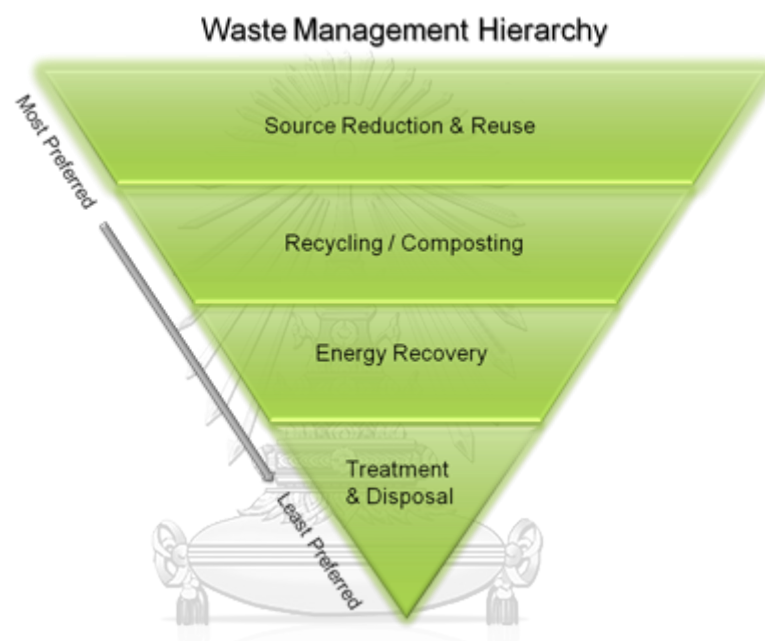
Figure 2.3 Integrated solid waste management hierarchy
