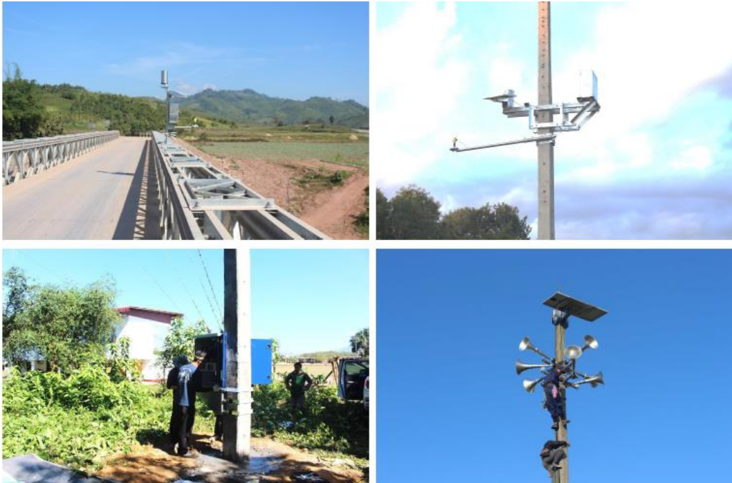
Figure 6.3: River water level measure, rainfall receive equipment, early warning system equipment and speakers in the Xay district
