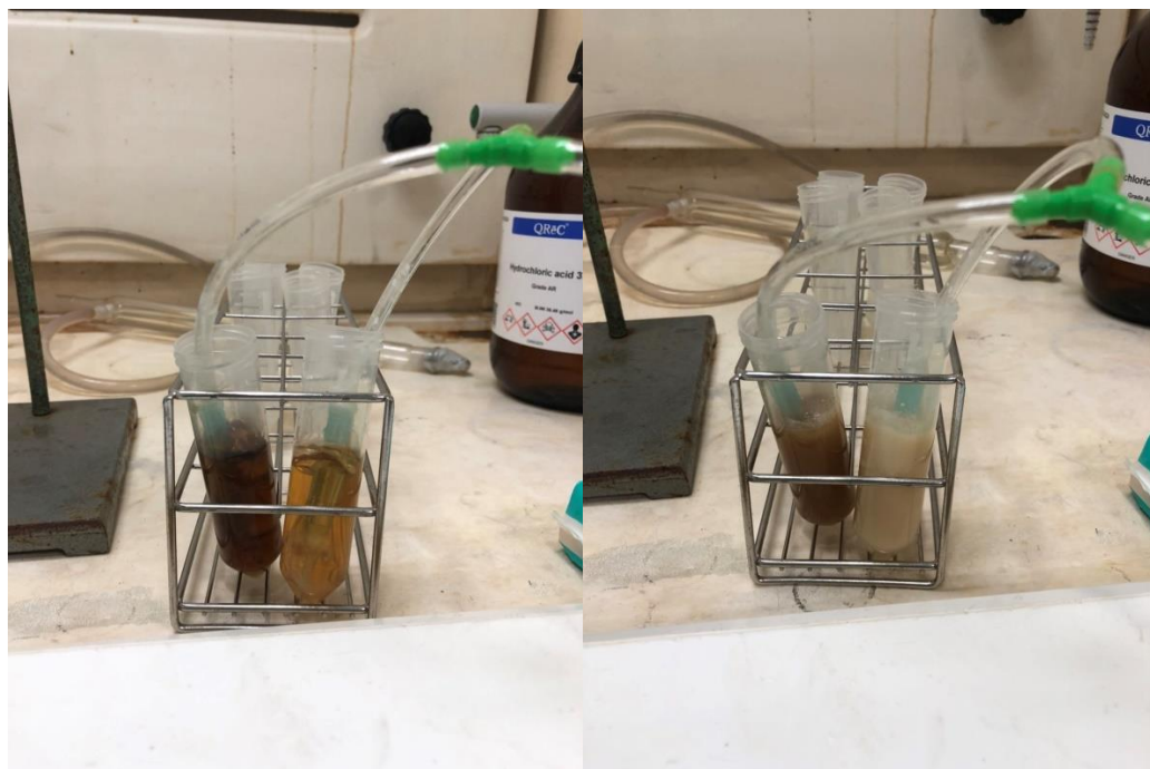
Figure 21. DBU conversion by \text{CO}_2 aeration process
