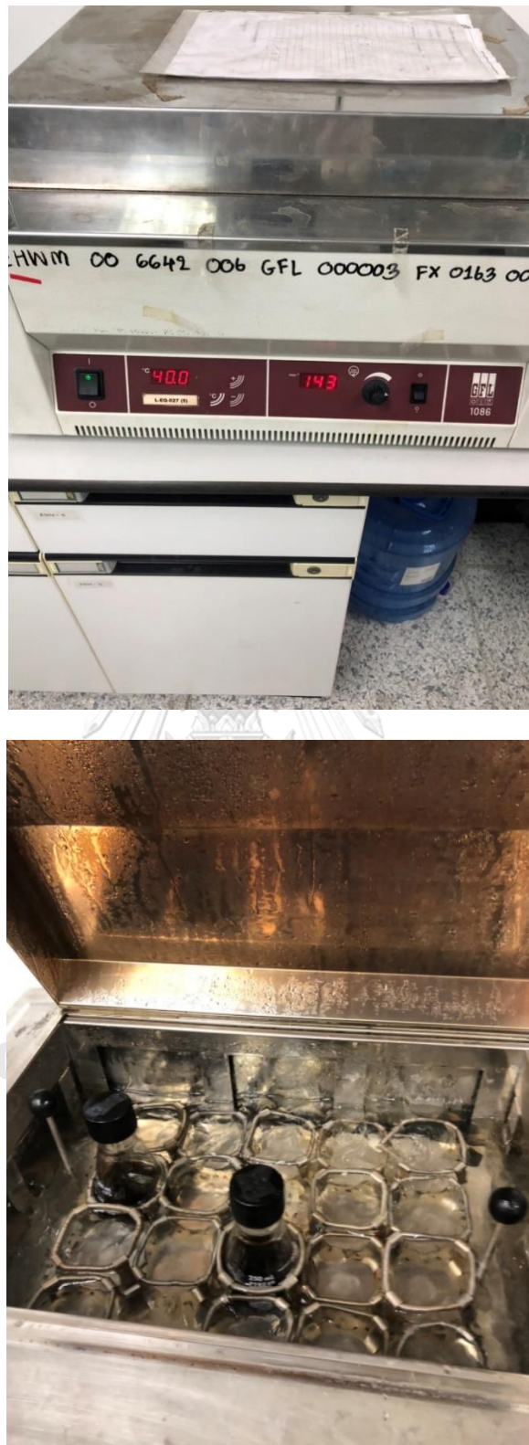
Figure 19. The in-situ TE process was performed in a water bath
