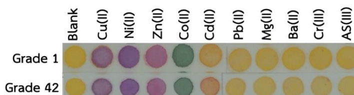
Figure 4.7 Color changes of PAN-metal complexes on device type A.
