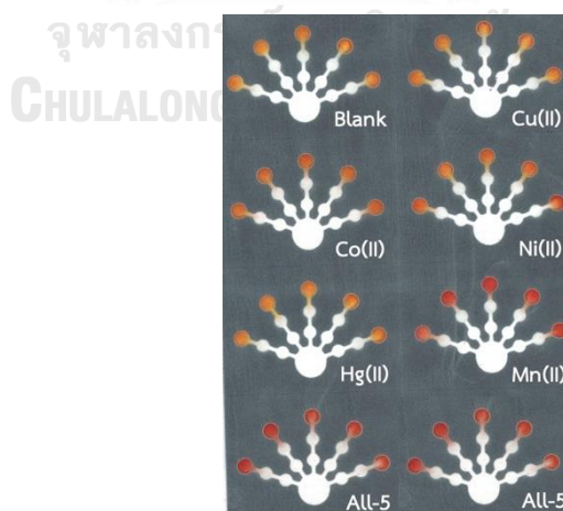
Figure 4.55 Color change of metal-PAR complexes on the device type F for Mn(II) detection.
