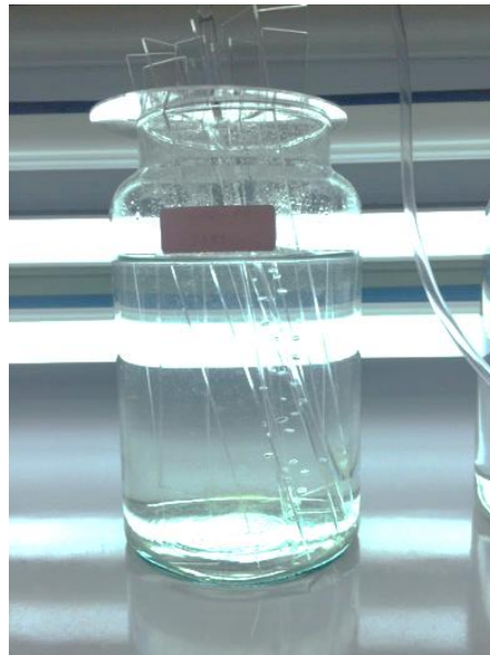
Figure 3 Amphora sp. growing bottle with 10 acrylic plates for diatom attachment.
