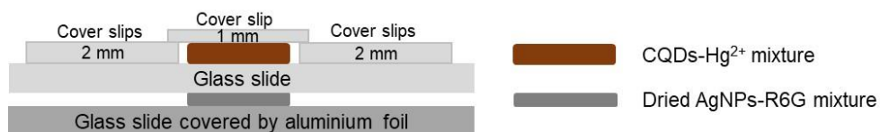
Figure 3.1 Schematic illustration of sample preparation for SERS measurement.
