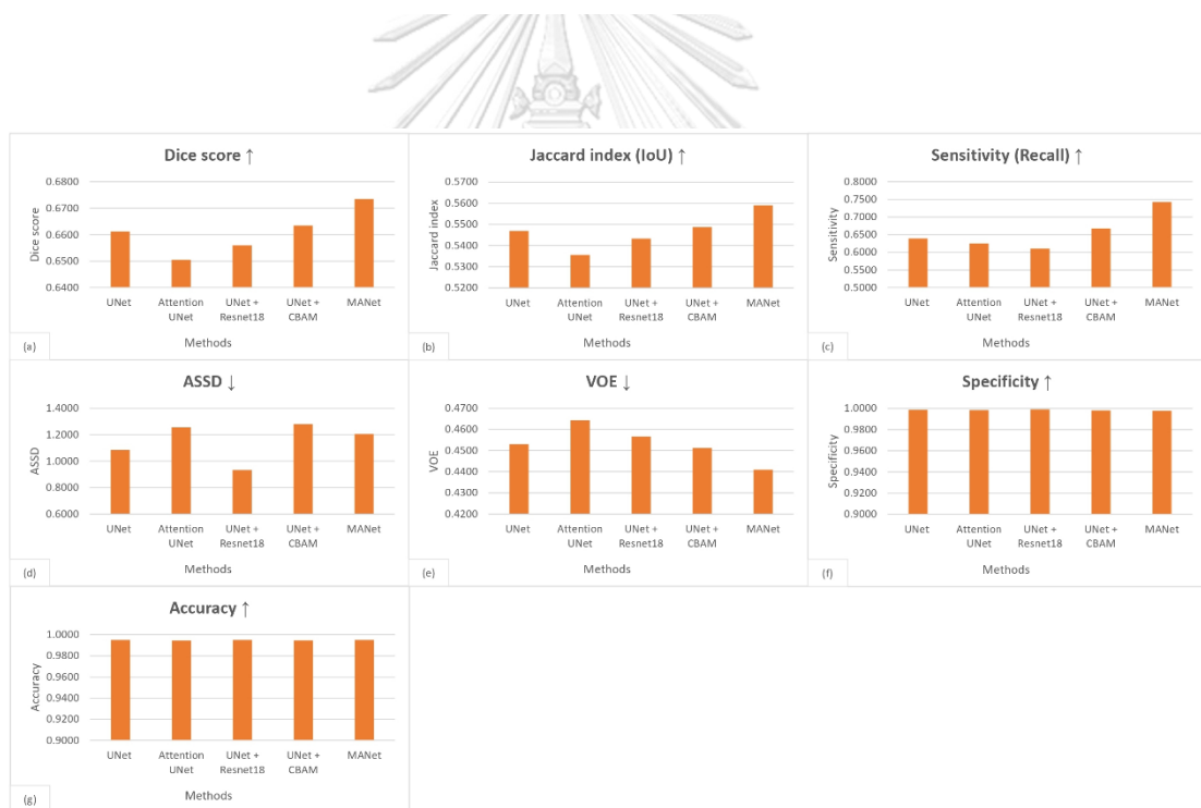
Figure 25: The quantitative liver tumor segmentation performance analysis of the proposed MANet model and the baseline models for volume-based segmentation on the LITS dataset for the measures:(a) Dice score, (b) Jaccard index (IoU), (c) Sensitivity (Recall), (d) ASSD, (e) VOE, (f) Specificity, (g) Accuracy.
