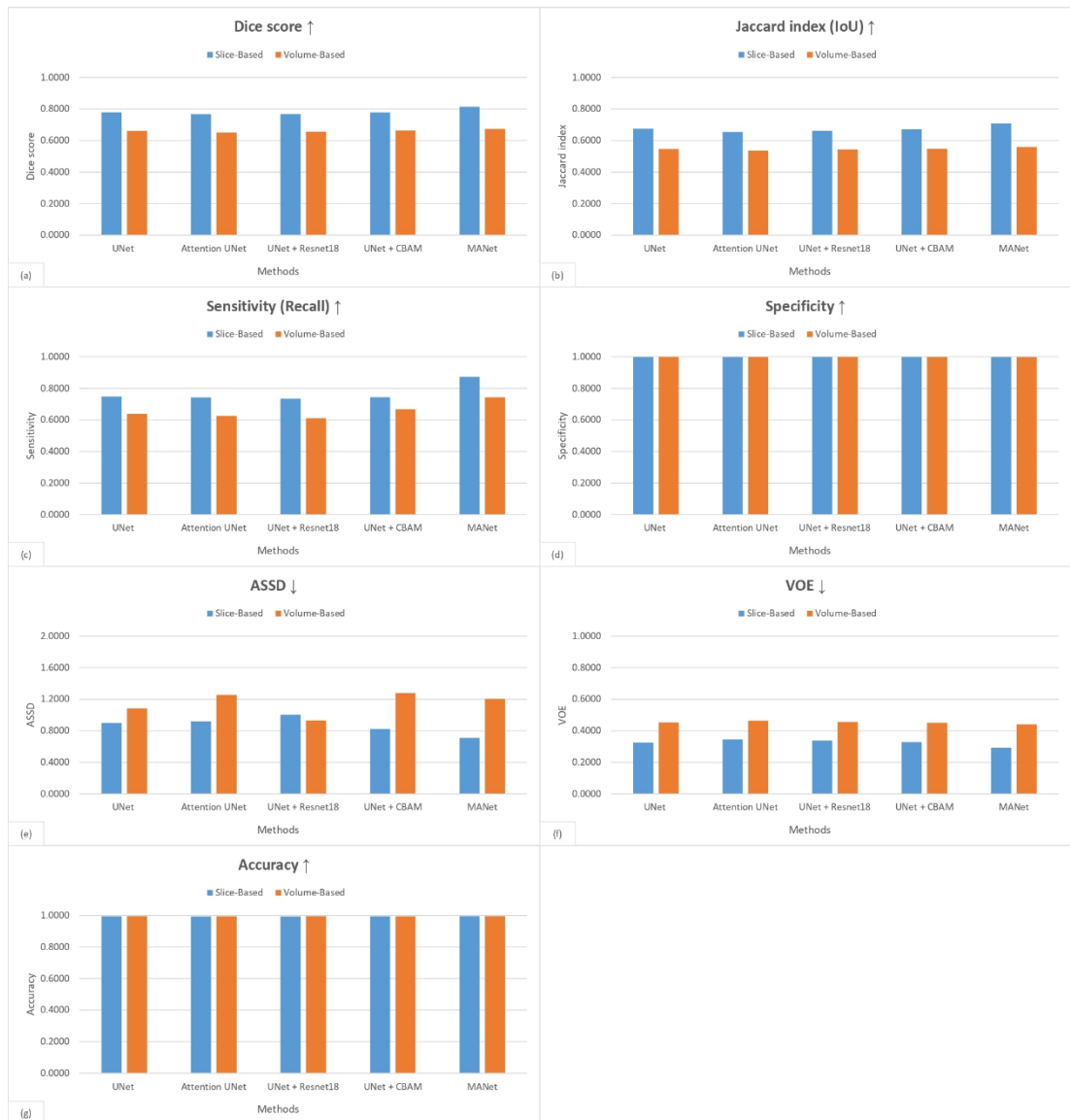
Figure 27: The quantitative liver tumor segmentation performance analysis of the proposed MANet model and the baseline models for volume-based and slice-based segmentation on the LITS dataset for the measures:(a) Dice score, (b) Jaccard index (IoU), (c) Sensitivity (Recall), (d) ASSD, (e) VOE, (f) Specificity, (g) Accuracy.
