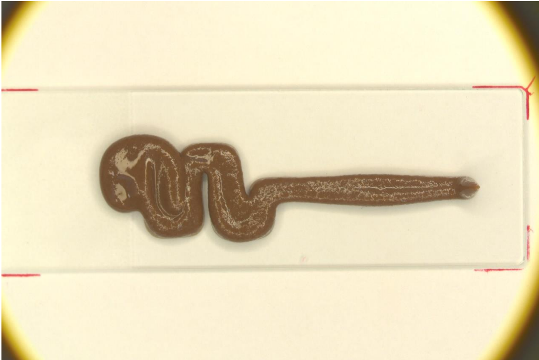
Figure 38 the result of chocolate fudge printing using pressure control mode at 10V (constant voltage input)
