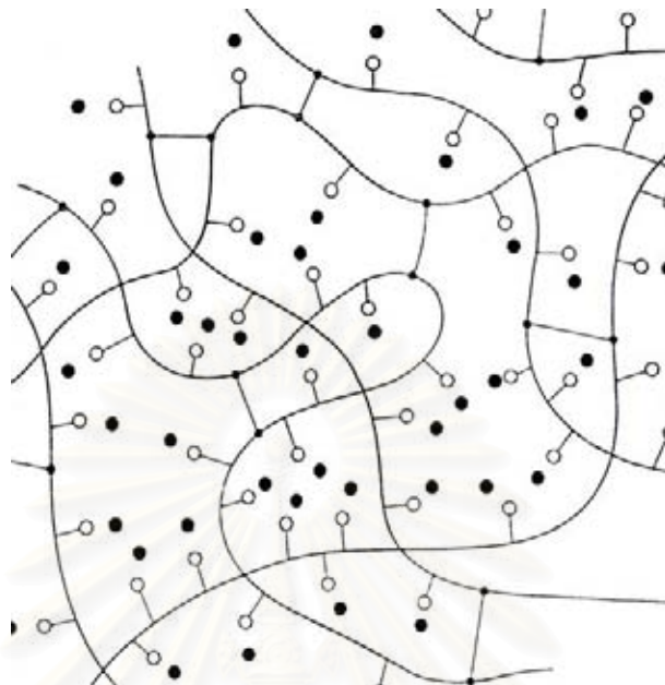
Figure 2 Schematic structure of ion exchange resins
