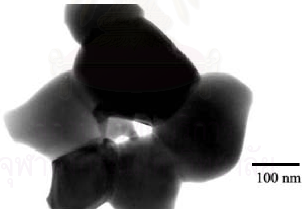
Figure 5.28(b) TEM photograph of zinc oxide synthesized at 200°C after calcined at 900°C (x100,000).
