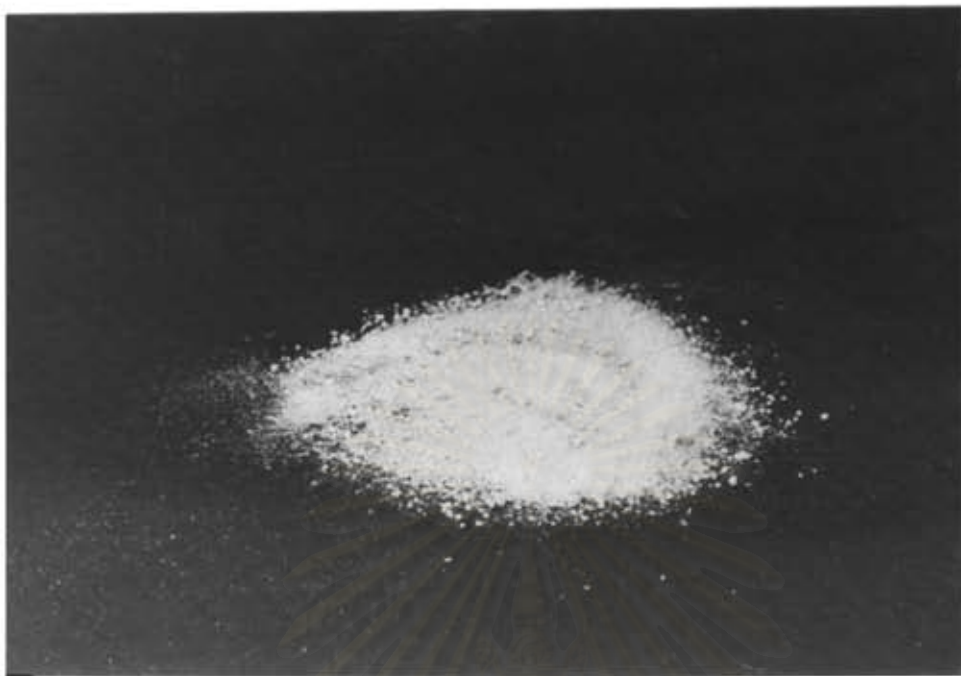
Figure 5.2 The glycolized product after EG extraction
