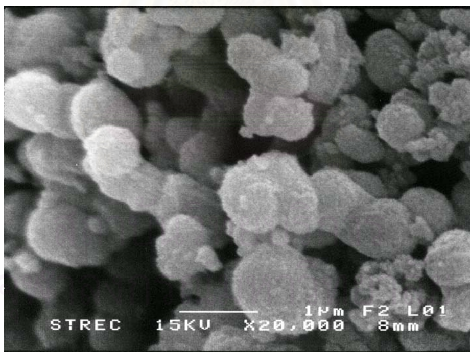
Figure 5.32: SEM images of alumina products: (a) as-synthesized product prepared in toluene, (b) product prepared in toluene calcined at 1180°C, (c) as-synthesized product prepared in mineral oil, (d) product prepared in mineral oil calcined at 1180°C.
