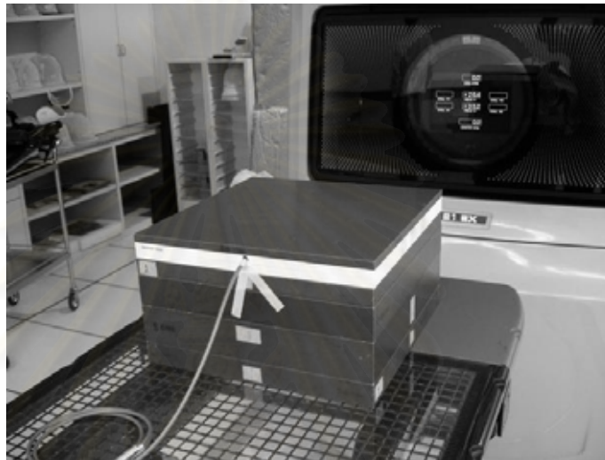
Figure 3.5 Solid water phantoms.
