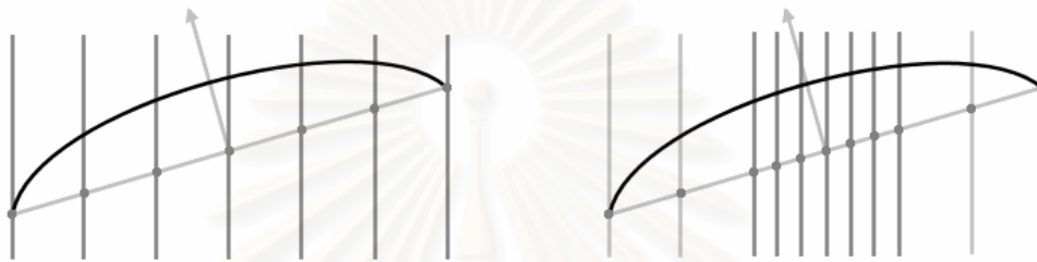
Figure 40. Determining the new midpoint of an edge
