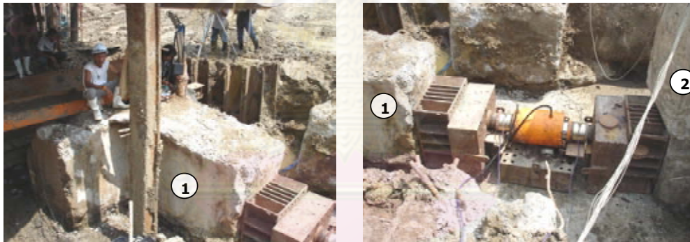
Figure 4.12 Layout for Static lateral load test on T-shape barrette with loading frame
