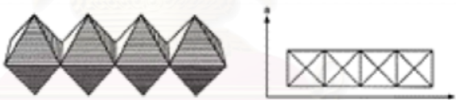
Figure 2.2 A diagram of rutile crystal structure
