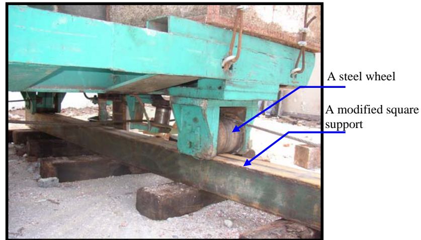
Figure 4.19 A support, a wheel and a wire rope of a pile-driving machine
