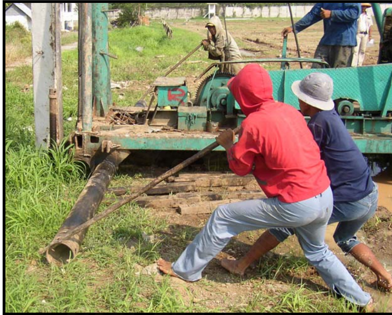
Figure 4.16 Mechanism of backward movement of Indonesian drop-hammer
