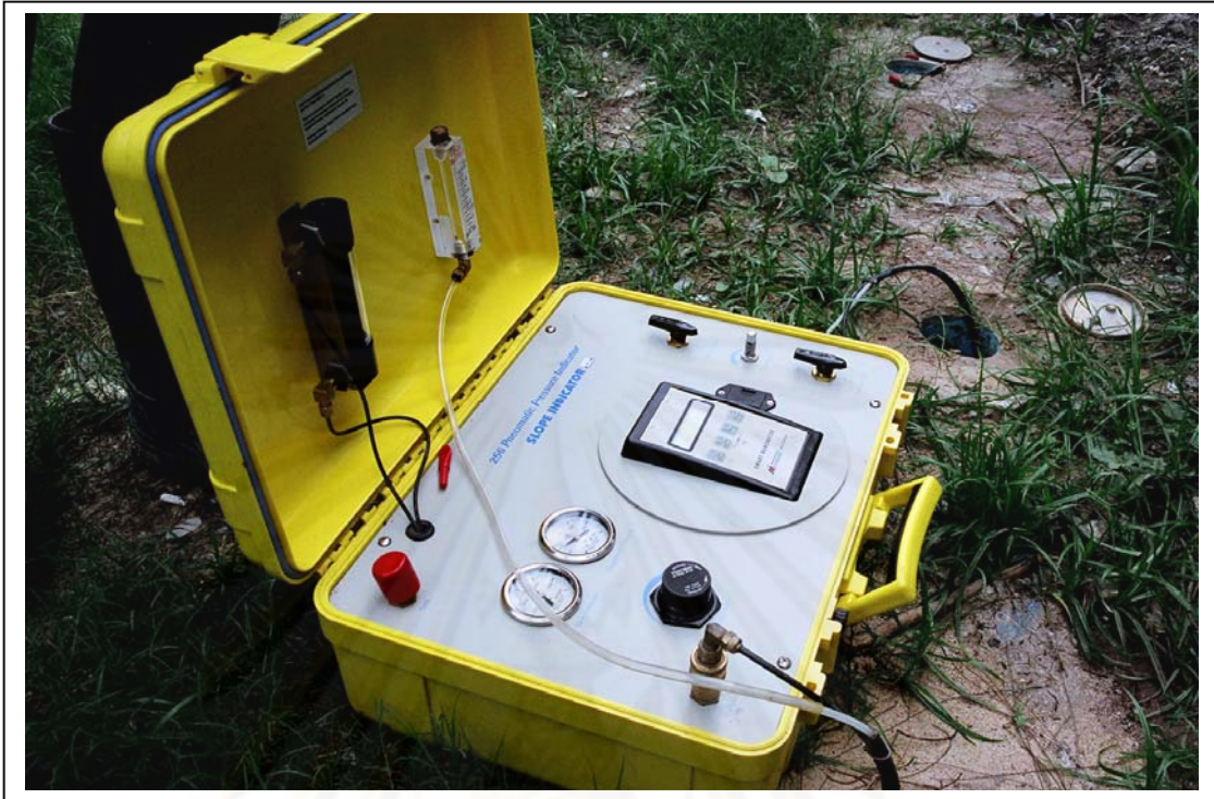
Figure 3.41 Monitoring equipment of pneumatic piezometer
