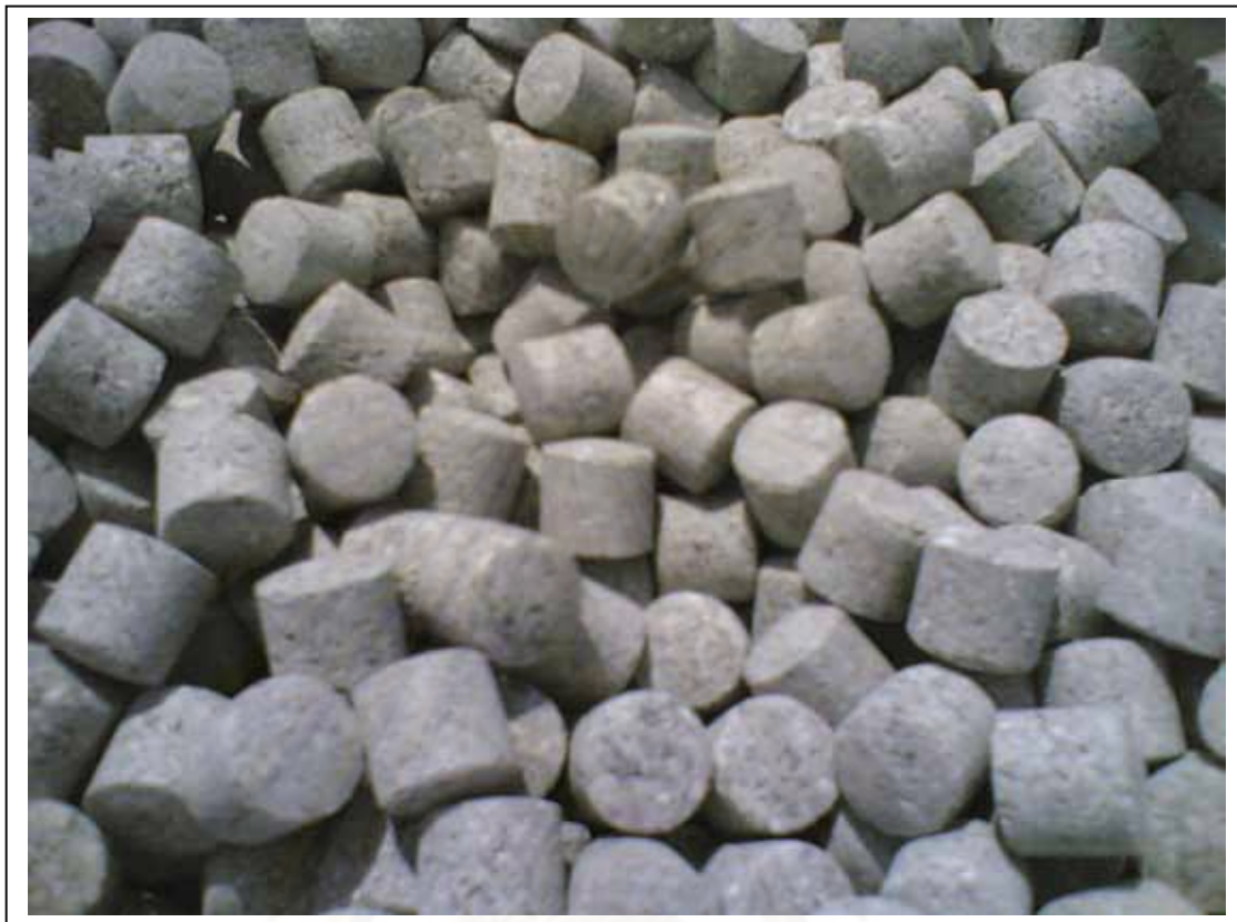
Figure 3.38 Palette bentonite used for piezometer installation
