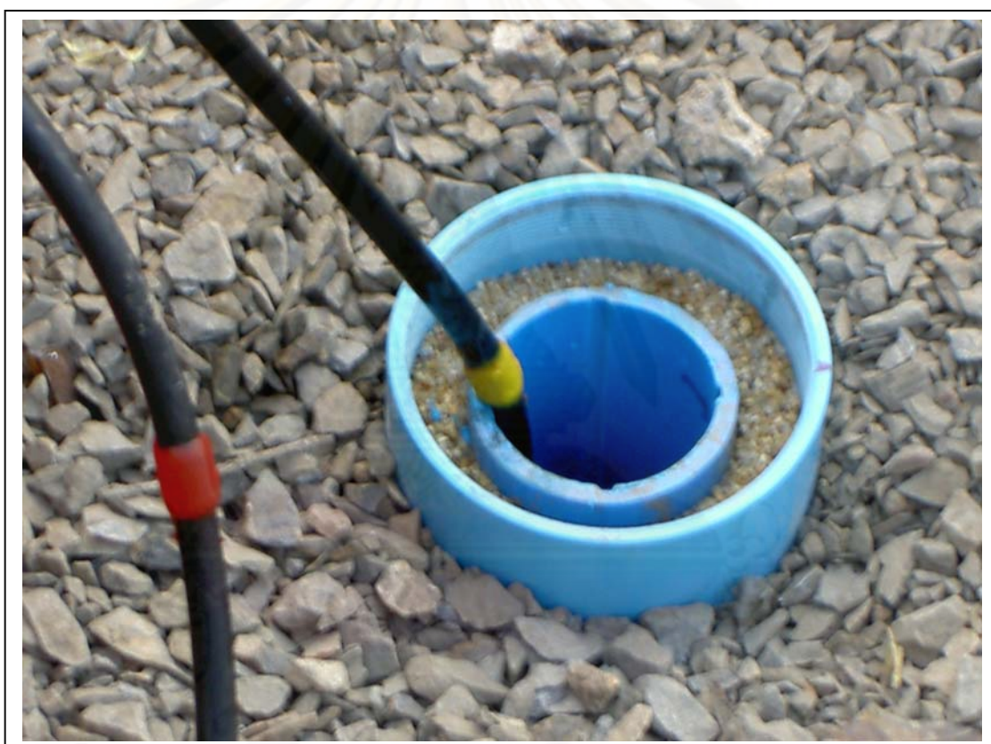
Figure 3.36 Yellow and red marks on the cable of inclinometer probe
