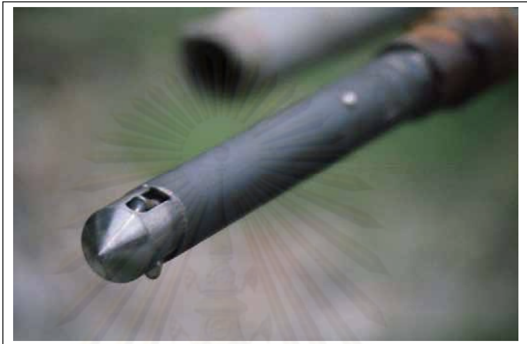
Figure 3.27 Prongs of deep settlement point
