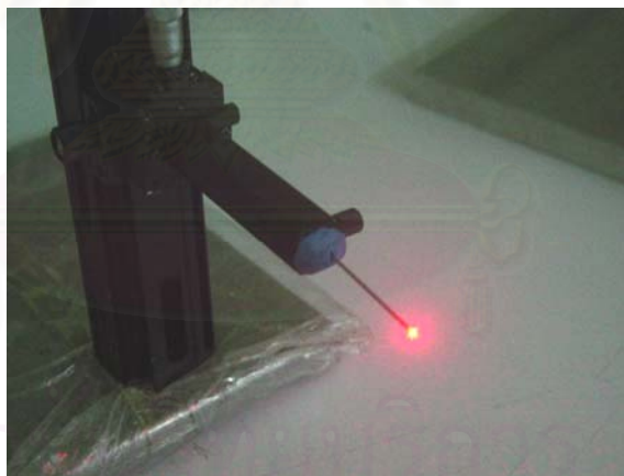
Figure 6.8 The photograph of the glass sphere attached to a thin pin at the measurement volume.
