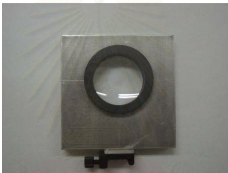
Figure 5.11 A symmetric-convex lens with 100 mm focal length and 50 mm in diameter.
