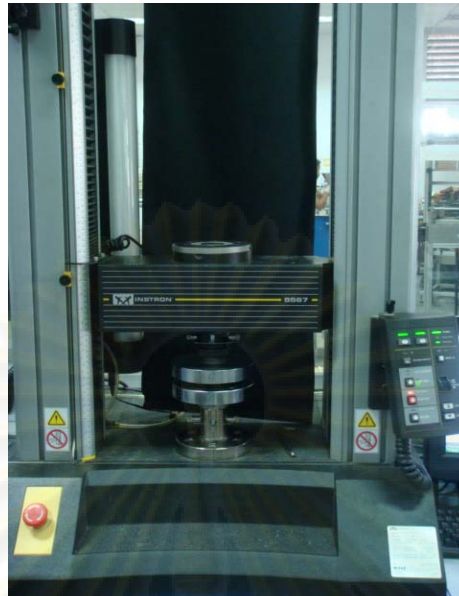
Figure 4.11 Universal Testing Machines (Instron Model 5567)
