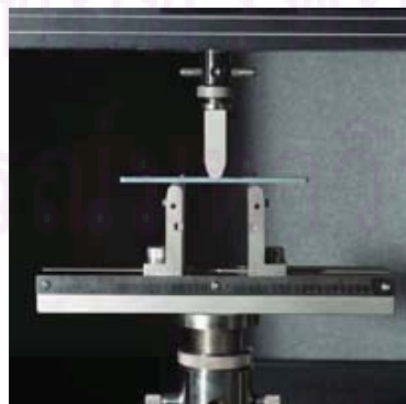
Figure 4.12 Universal Testing Machines (Instron Model T609-109) for Flexural Test [33]
