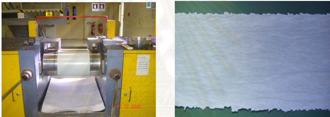
Figure 4.3 PVC stock / glass fiber compound from a Two-roll Mills
