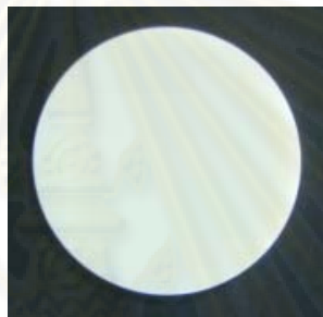
Figure 4.6 Specimen (disk) for Water Absorption evaluation
