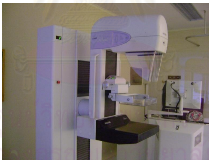
Figure 3.1 The FFDM Hologic, LORAD model Selenia system with Molybdenum and Rhodium targets.
