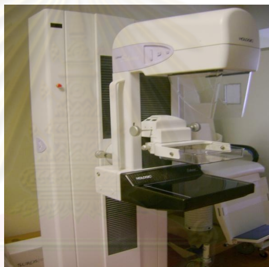
Figure 3.2 The FFDM Hologic, LORAD model Selenia system with Tungsten and Rhodium targets
