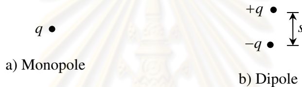
Figure 2.1: Physical interpretation of a monopole and a dipole in space.
