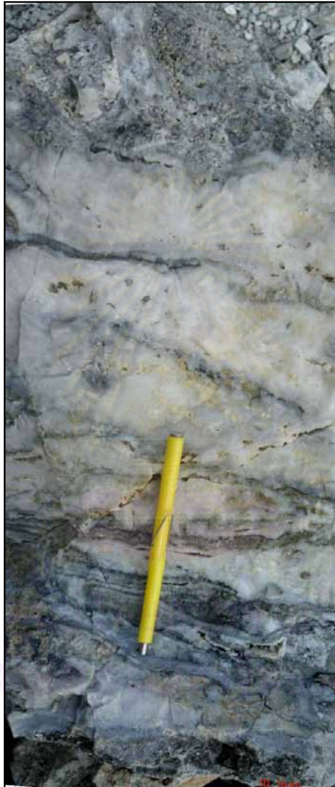
Figure 4.11 Photograph of Stage III core sample showing alternating quartz–carbonate with sulphide bands and chalcedonic bands.
