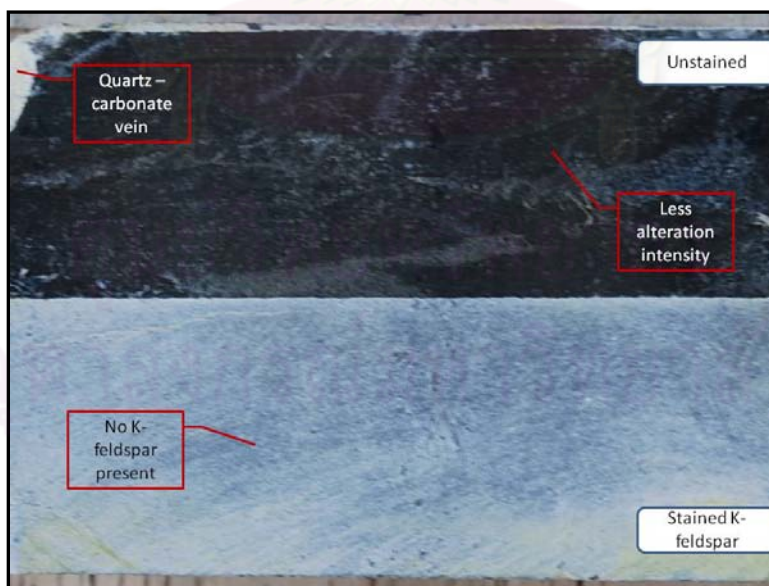
Figure 3. 42 Photograph of andesitic rock (unit 3) showing slight alteration and few crosscutting quartz-carbonate vein without K-feldspar (stained slab).
