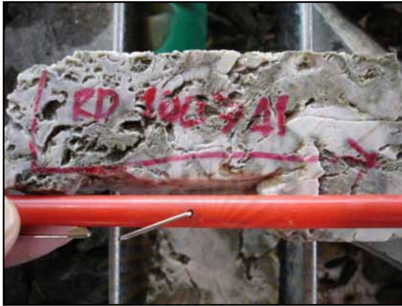
Figure 4.12 Photograph of Stage III core sample showing carbonate leached out from quartz – carbonate – chalcedony vein.
