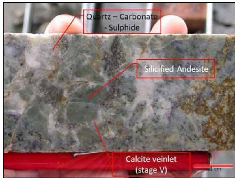
Figure 4.16 Photograph of core slab showing Stage III quartz-carbonate-sulphide minerals cementing silicified andesite clasts, and later crosscut by calcite veinlets (Stage V).
