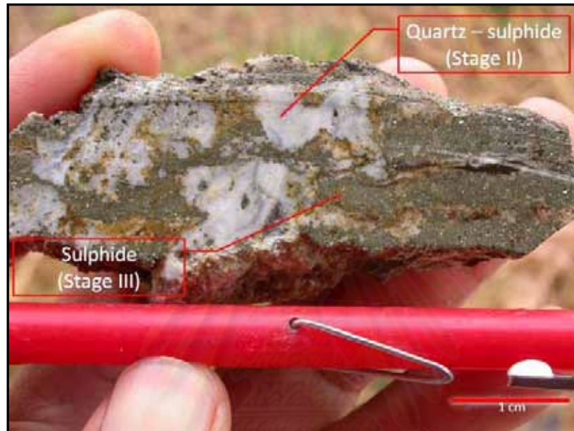
Figure 4.10 Photograph of core sample showing quartz-euhedral pyrite (Stage II) clasts embedded in sulphide-rich veins (Stage III).
