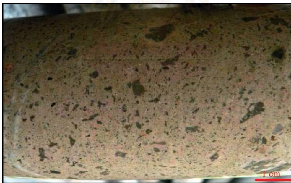
Figure 3. 19 Photograph of core sample displaying completely chlorite-replaced-fiamme clasts of the fiamme unit.
