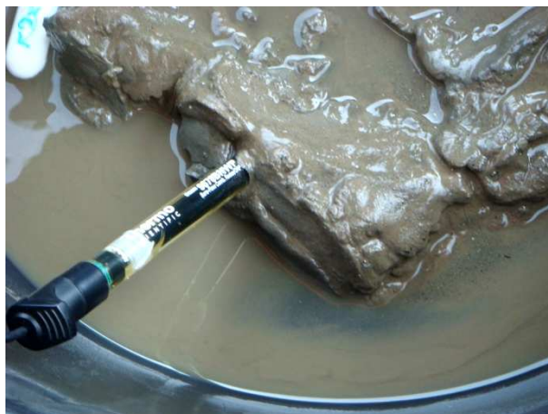
Figure 3-7 Measurement of redox potential (Eh) using Platinum Combination Redox Electrode (Thermo Orion 290A)
