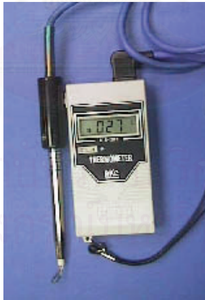
Figure 3.5 Thermometer used for the mould surface temperature measurement.
