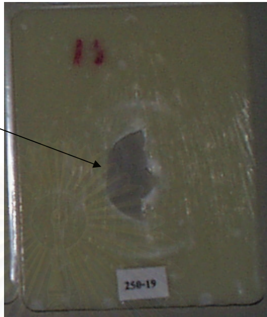
Figure 4.27 Cracked specimens of ABS Lustran 250 moulded at melt temperature of 280 °C.
