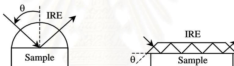
**Figure 2.5** IRE configurations commonly used in ATR experiments: single reflection variable-angle hemispherical crystal (left); and multiple reflection single-pass crystal (right).
